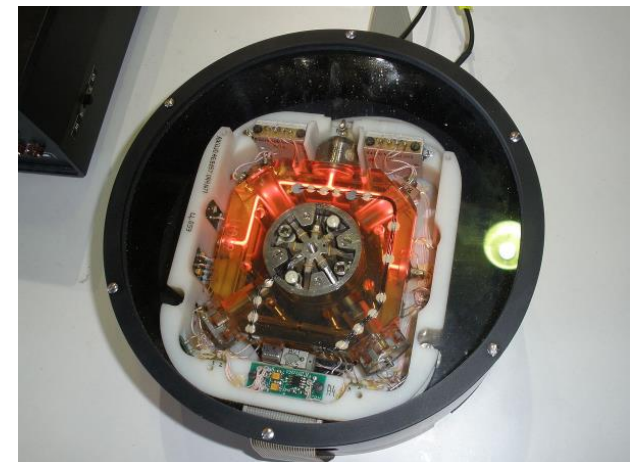
Image: “Ring laser gyroscope produced by Ukrainian “Arsenal” factory on display at MAKS-2011 airshow#, by James Nockson
