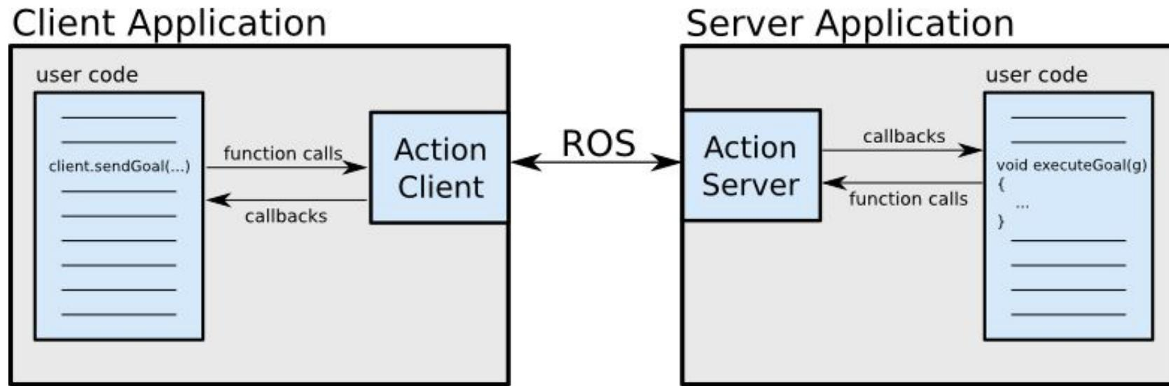
The ActionClient and ActionServer communicate via a "ROS Action Protocol", which is built on top of ROS messages
