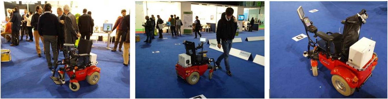
Fig. 8. LURCH at Robotica 2010. From left to right: typical crowded moment, with LURCH moving among visitors; LURCH modifying its trajectory to avoid a fast moving passer by; back view of LURCH, showing the special configuration used for the fair (downward looking camera, self localization markers fitted to the floor).
