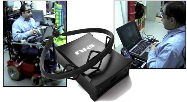
Fig. 6. The electro miographic interface based on the NIA gaming device.
