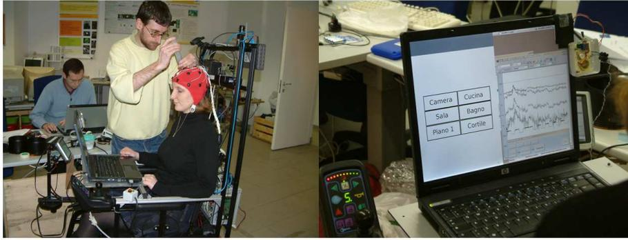
Fig. 7. The Brain-Computer Interface setting on the LURCH autonomous wheelchair; on the left the electrodes setup, on the right the acquisition of brain signals.
