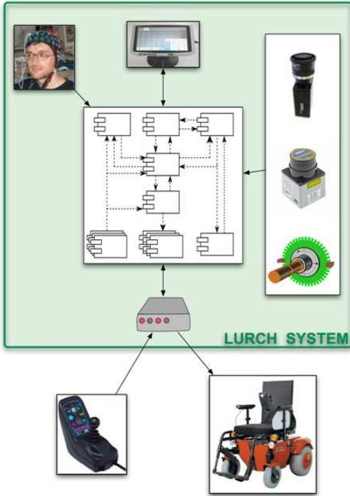
Fig. 2. The LURCH architecture; the control system is independent from the wheelchair, and the gateway between LURCH and the vehicle is represented by an electronic board that intercepts the analog signals coming from the joystick potentiometers and generates new analog signals to the wheelchair. Sensors used by LURCH are low-cost laser range finders, wheel encoders, and an upward looking camera.
