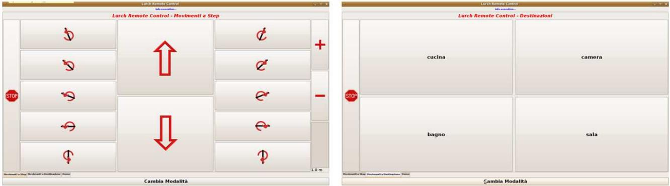
Fig. 5. The two modalities for the touch-screen interface: command mode (on the left) and destination mode (on the right).
