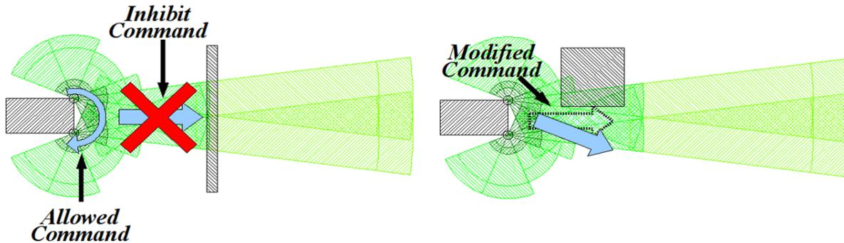
Fig. 4. By the use of a set of fuzzy rules it is possible to implement avoid strategies when facing unexpected obstacle.
