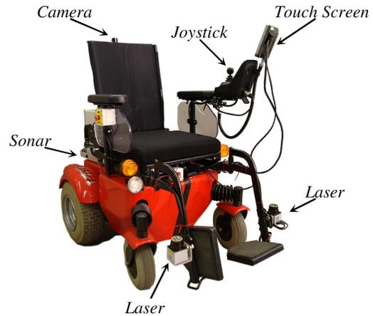
Fig. 1. The LURCH autonomous wheelchair equipped with sensors for autonomous navigation and the touch-screen interface.
