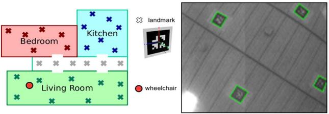
Fig. 3. A set of passive markers (in the middle) is placed on the ceiling of the environment to provide a global localization system (on the left) through the upward looking vision system (on the right).
