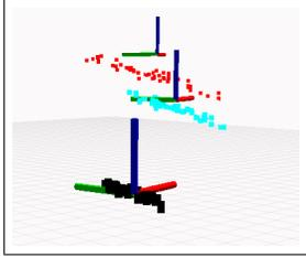
Fig. 8. 3D view of the particle set for the naive motion model. Notice that the larger the overall  $\Delta y_{aw}$  and  $\Delta z$ , the larger the distortion of the particle set.
