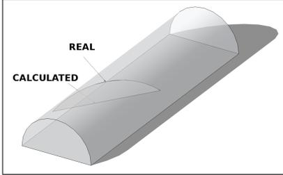
Fig. 4. REAL and CALCULATED (basing on odometry) trajectories, which impact on the uncertainty on  $\delta_{transl}$ , as due to a change in roll ( $\Delta\varphi$ ).
