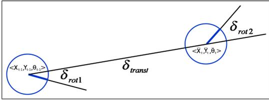
Fig. 1. 2D-3DoF motion model from [2, Sect. 5.4].
