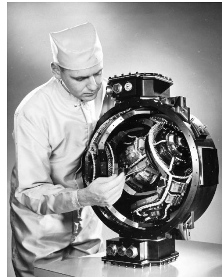
ST-124 Inertial Guidance Platform used in the Saturn V, 1960s
