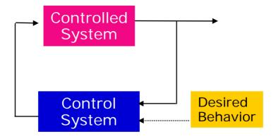
In most cases it is a PID controller, where the output  $\boldsymbol{u}$  depends on the difference e between the desired, and the observed behavior, its derivative (how fast  $\boldsymbol{e}$  changes) and its integral (how large  $\boldsymbol{e}$  has been in the past):
