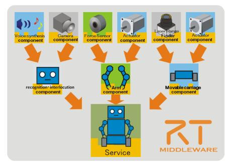
OpenRTM-aist (Advanced Industrial Science & Technology) is based on the CORBA technology to implement RTC extended specification
